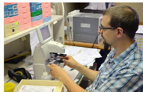
ABOVE: Florian Peter, a prescription eyeglass maker inspector, does a quality assurance check on a set of new prescription glasses produced at the U.S. Army Medical Materiel Center-Europe’s optical fabrication lab. (Photo by Lt. Col. Marc Welde)
