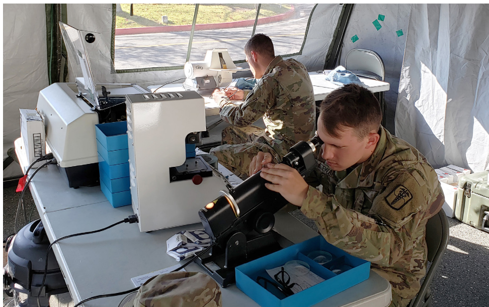
ABOVE: Florian Peter, a prescription eyeglass maker inspector, does a quality assurance check on a set of new prescription glasses produced at the U.S. Army Medical Materiel Center-Europe’s optical fabrication lab. (Photo by Lt. Col. Marc Welde)
